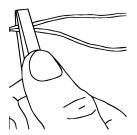
Cut the end of the cord that protrudes from the guide channel #1 or #5 at approx. 30cm cord length overhang with a cutter. The cut surface must not be frayed when cutting through. A swift cut with moderate pressure works better with Dyneema than light sawing movements.
