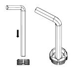
Place the Nut Cap onto a table as illustrated Remove the Hex Key and place the nut in and insert in the Hex Key in it. A little the Nut Cap. pressure might be needed.
