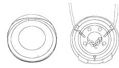
The base has two recesses that branch away from the cords and one recess that points towards the cords. The 'atop' itself has one protruding edge on the side through which you have inserted the strings and two protruding edges on the opposite side.
