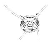
Insert one end of each cord over the outside into the respective cable duct. The cord end should come out on the inside or underside of the 'atop'. Be sure to insert the cords into the correct holes by holding the 'atop' against its base in the socket, checking which cord end goes to which hole.
