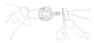
Use combination pliers to grab the respective loose end of the cord. Use your other hand to grab the long end of the cord sticking out of the 'atop'. Now tighten the two knots individually or simultaneously. Cut off the excess end of the cord.
