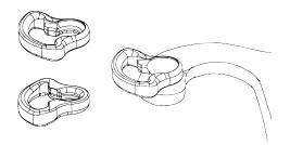
Take the two Velcro loops. These are attached to the outer end of the condylar braces.
