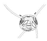
Insert one end of each cord over the outside into the respective cable duct. The cord end should come out on the inside or underside of the 'atop'. Be sure to insert the cords into the correct holes by holding the 'atop' against its base in the socket, checking which cord end goes to which hole.
