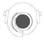
Position the padding washer inside the socket (shown here in black). Make sure that the disc remains in the desired position. Check one more time from the other side that no adhesive is visible through the hexagonal hole.
