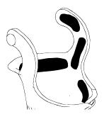
Cut out two approx. 1x1cm pieces of the selfadhesive Velcro material. Round off the edges. Stick one of each of these two pieces on the inside of the condylar braces.
