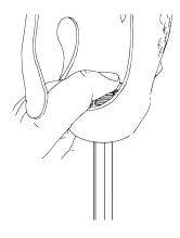
With your finger, press the Nut Cap with the nut inside against the threaded hole in the socket from the inside while you insert the Hex Key into the hex hole of the nut cap through the round distal hole of the socket. If the socket is long, a tool can be used instead (like the handle of a hammer).
