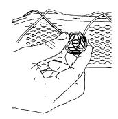
Anchor the 'atop' in the atop base. First, push the two protruding edges of the 'atop' rim into the recesses provided. Then press the entire 'atop' into the base.
